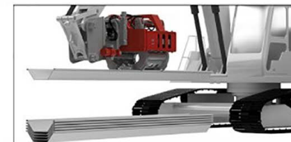
Carrying Sheet Piles
